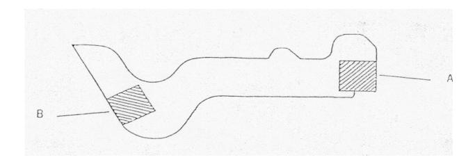
Figure 1: Angle guide plate: removal positions A and B for test specimens for the impact strength test (DIN EN ISO 179-1). When performing the test, the unmachined side of the test specimens is to be placed in the tensile zone. The test specimens for the test of tensile modulus of elasticity shall also be taken from the areas around A and B (DIN EN 527-2)
