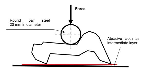
Figure 2: Angle guide plate: principle of the bending test on the finished part
